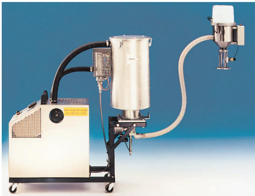
When processing hygroscopic plastic materials for technical products, it is important to have the best marginal conditions for optimum of quality. Particulary when supplying processing machines with small throughputs, the drying results are often reduced by external influences.
